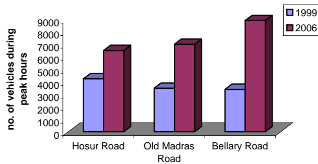
Figure 4.6 Change in peak traffic flow volumes on three of the major intercity corridors for Bangalore - 1999 and 2006
