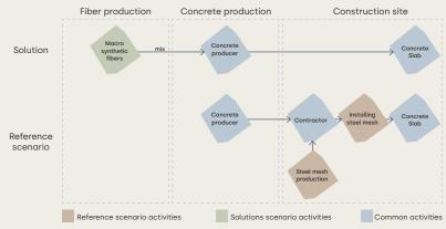
Offers a lower carbon solution to reduce Scope 3 of contractors and construction
